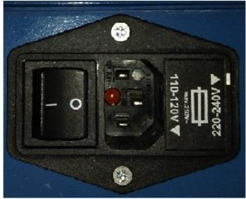
*Figure 5: IEC Connector on Back of Surface Box set up for a voltage input of 220 - 240V AC*
