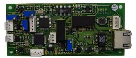
Figure 12: Ethernet Board Top Side
