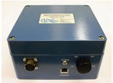
Figure 4: Ethernet Surface Box
